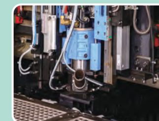
盲鑽、背鑽加工機能 Depth drilling / Back drilling Function
